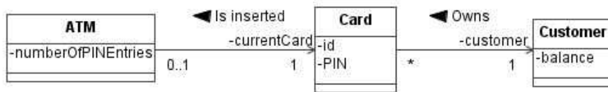
Fig. 3. Class diagram (Domain model) of the ATM.
